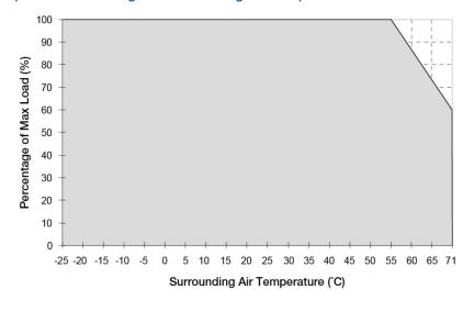
Fig. 1 De-rating for Vertical Mounting Orientation > 55°C de-rate power by 2.5% / °C
