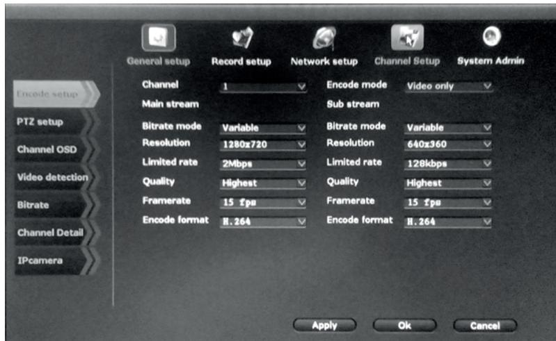
**Encode setup** – sets up quality of the given channel
