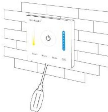
Plug into the below bayonet with a screwdriver,
