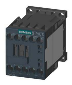
CONTACTOR, AC-3, 5.5KW/400V, 1NO, DC 24V, 3-POLE, SZ S00 SCREW TERMINAL .
