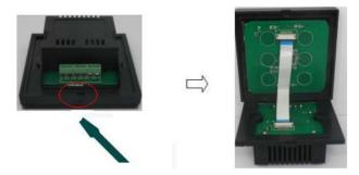
(2) as shown in figure: the flat cable taken down. Open the lock connection seat, take the flat cable
